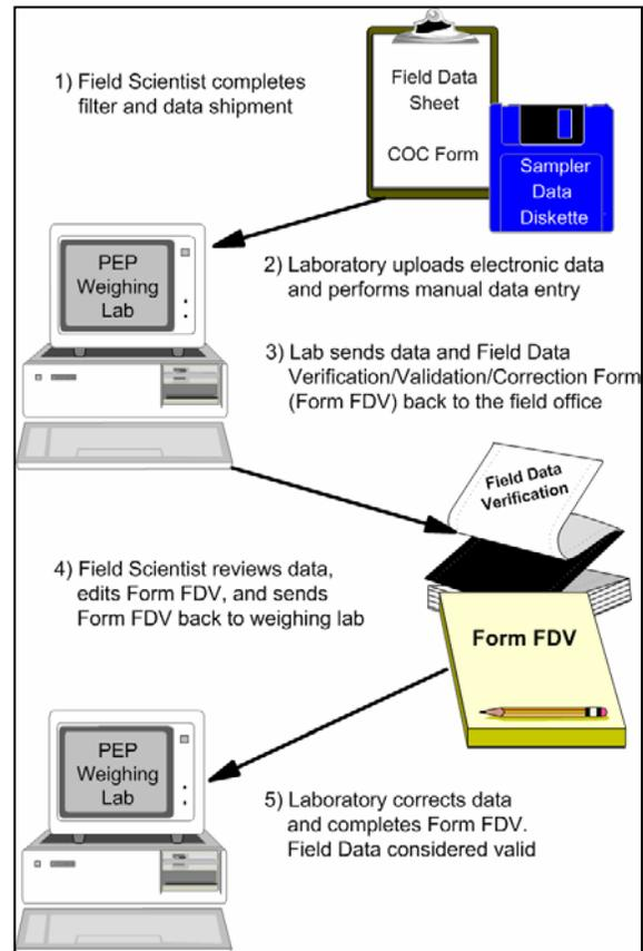
**Figure 8-2. Field data verification/validation flow.**
